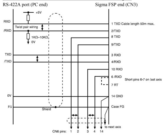
Pins 6-7: Short to use an internal terminating resistor (see table below).
